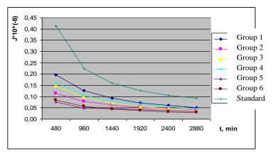
**Fig. 4** Wear intensity of the "standard" sample and the samples with two identical weld overlaid layers in a dry abrasive environment, made of the K16 molding mixture
