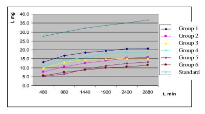
**Fig. 2** Dynamics of the wear magnitude of the "standard" sample and the samples with two identical weld overlaid layers in a dry abrasive environment, made of the K16 moulding mixture
