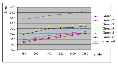
**Fig. 3** Dynamics of the wear magnitude of the "standard" sample and the samples with two identical weld overlaid layers in a wet abrasive environment, made of the K16 molding mixture
