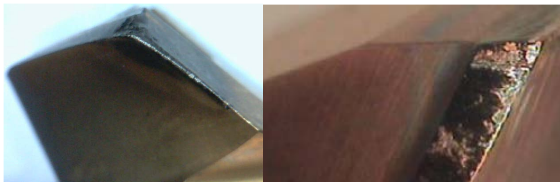
Fig. 7 Wear of the cutting edge – chipping of the edge (left) and flank wear (right)
