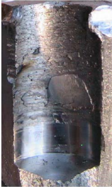
Fig. 1 Surface of the hole drilled without cooling – steel 11 523
