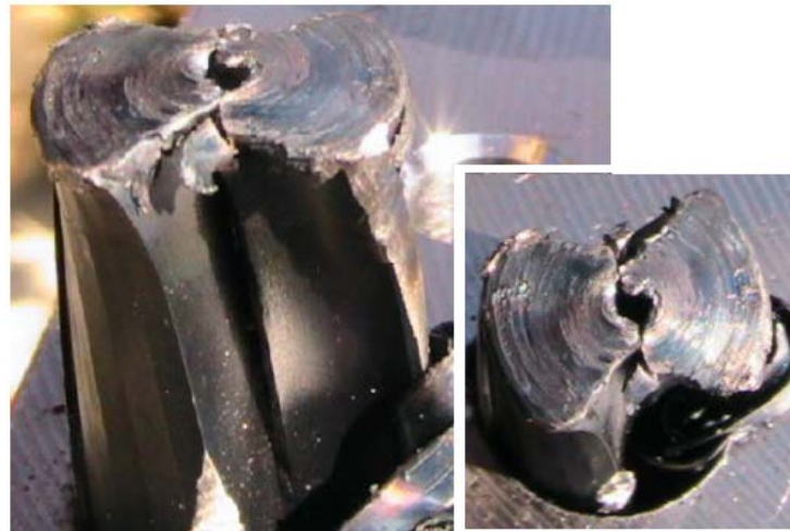
Fig. 2 Longitudinal crack of body caused by the reduced cross-section of the body core
