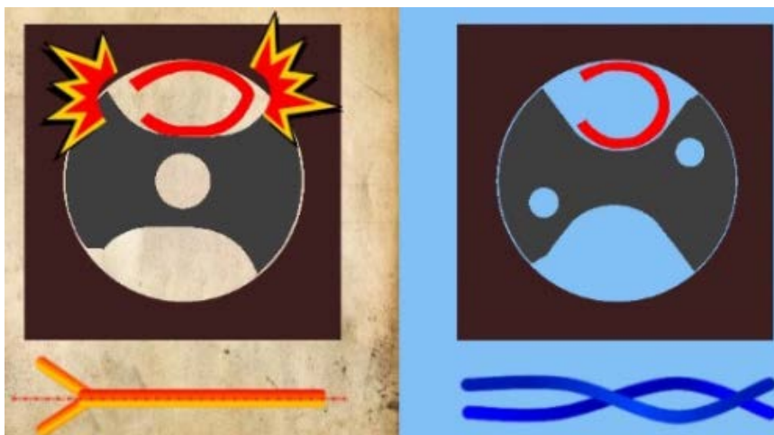
Fig. 3 Comparison of single (left) and double (right) cooling channel design and its impact on flute cross-section size [5]
