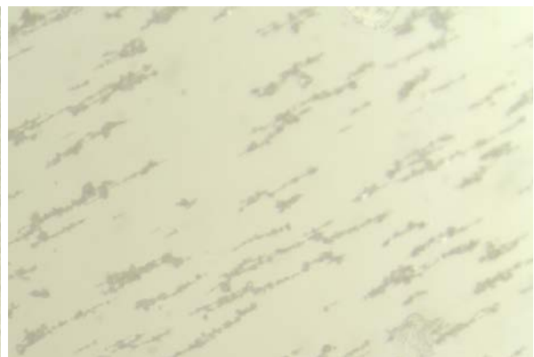
Fig. 3 Wear particles in fluid after 450 engine hours
