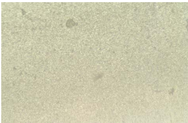
Fig. 2 Wear particles in a new fluid
