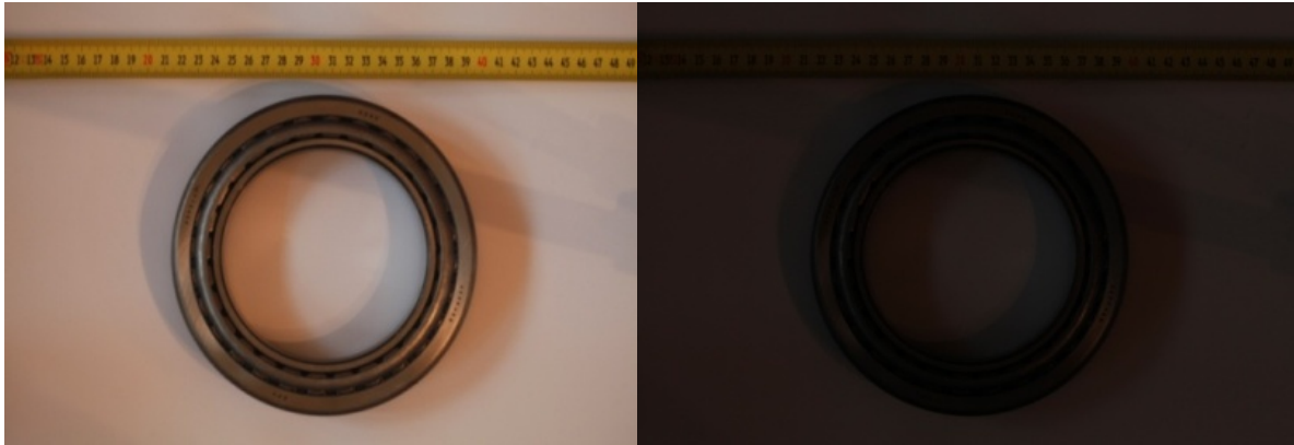
Fig. 3-4 Effect of aperture value to photo quality
