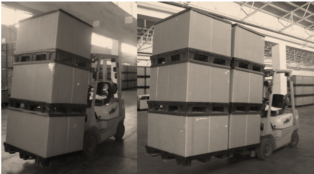
Fig. 4 The use of traditional and extended forks in the store of SKOB enterprise
