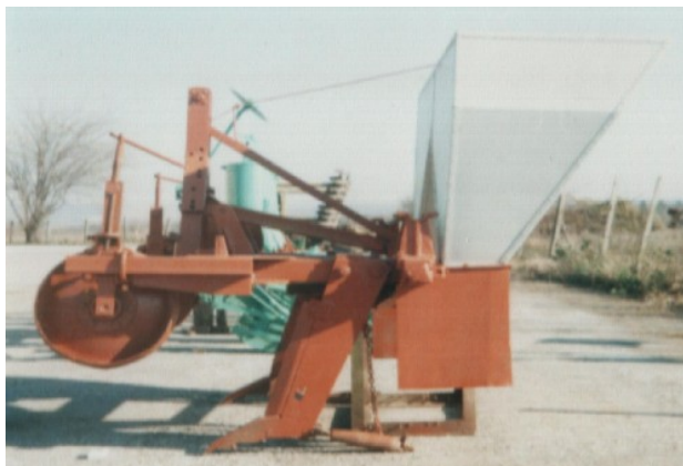
Fig.1 Reconstructed breaker-dead furrower ИЦН 2-140 for making soil slots, with bunker for mulch
