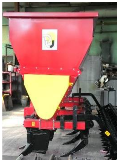
Fig. 2 Device for depositing mulch or organic matter in the soil
