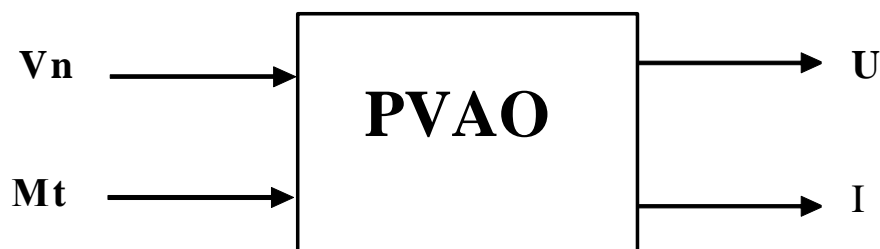
Fig.1 Cybernetic model of vibrating arc overlaying process (PVAO) in a shield of Ar:
