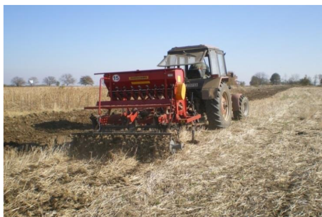
Fig. 1 Overview of sowing aggregate "Belarus 952" and cultivator drill SCS – 2
