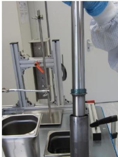
Fig. 5 Disassembly of the piston rod out of the cylinder tube
