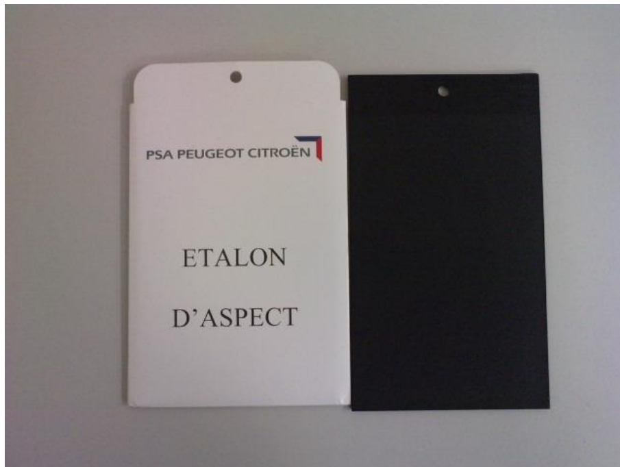
Fig. 1 Standard for gloss check
