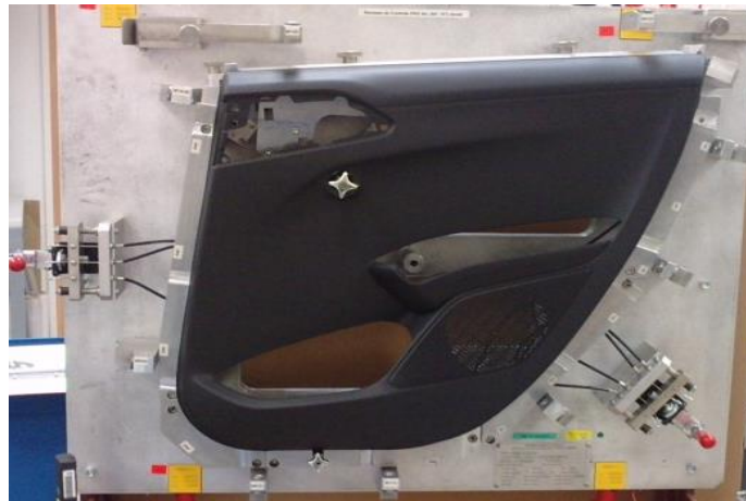
Fig. 3 ARD 91 rear carrier clamped in a measurement preparation
