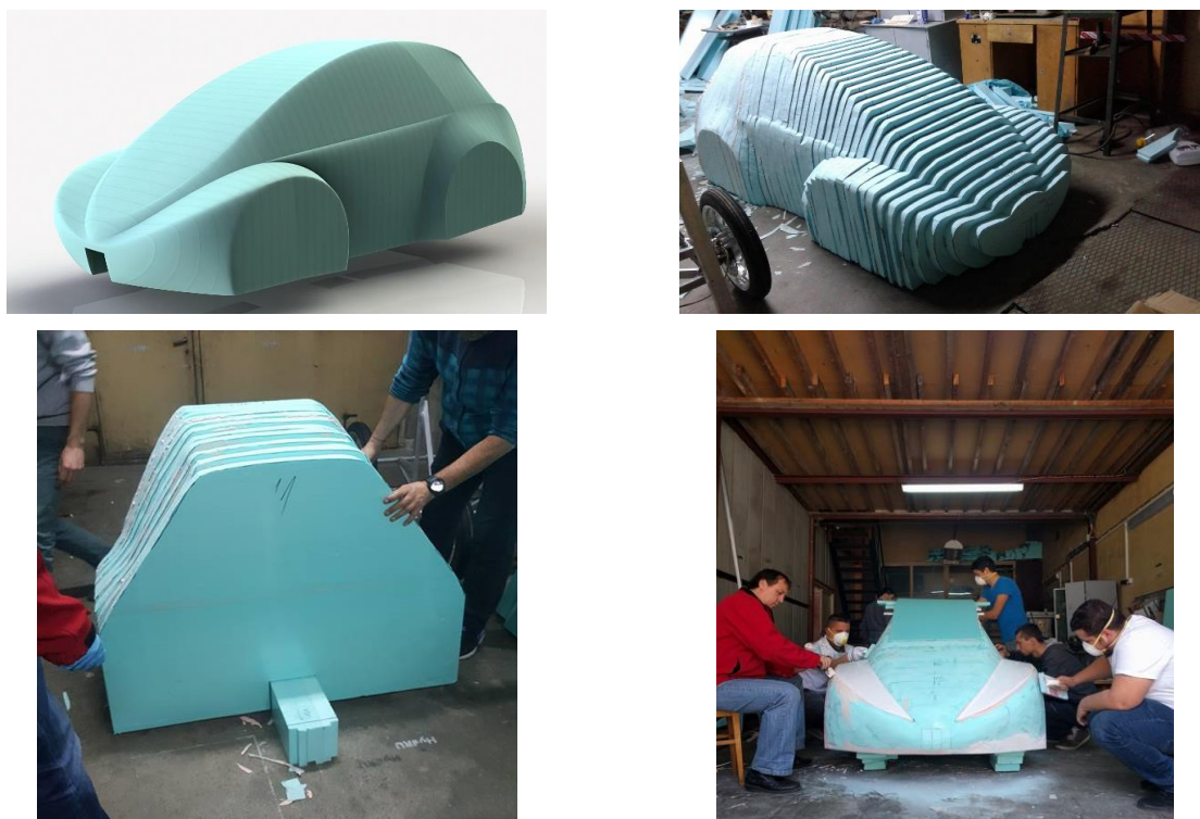
Fig. 3 Different stages of the modelling using the vertical sections of the car made from XPS
