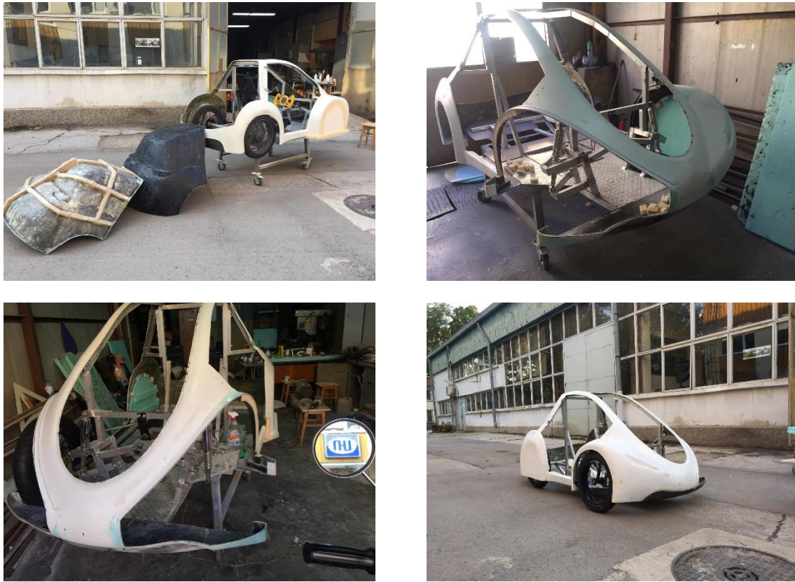
Fig. 8 The initial prototype of the vehicle was cut and the parts were used to make moulds and cast the new body components
