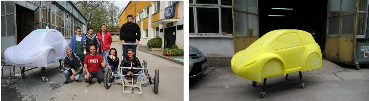
Fig. 4 The team after the sanding of the vehicle model and the car after the isolation material was applied
