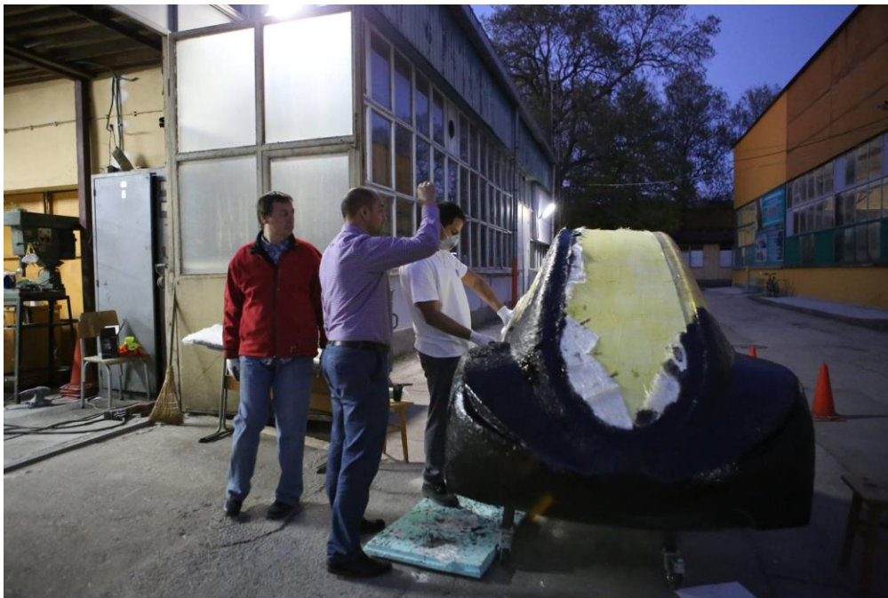
Fig. 5 Part of the team while applying layers of resin and fibre cloth to the vehicle model. Due to the specifics of the process and the requirement for the drying of the resin, we had to work even till very late in the night
