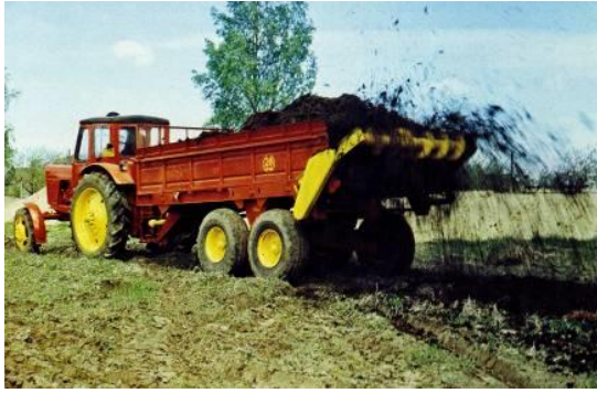
Fig. 1 Fertilizer spread trailer 1PTU – 6
