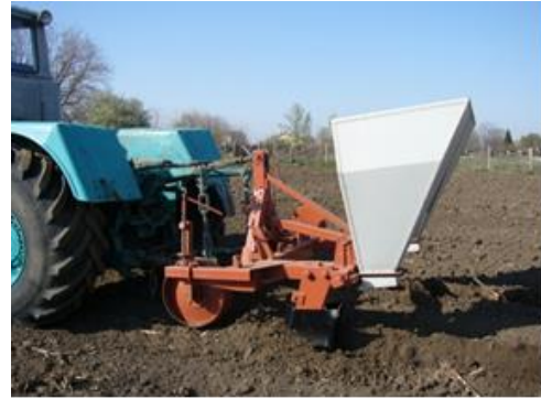
Fig. 2 Machine for vertical mulching SHTN 2- 140 with bunker for mulch
