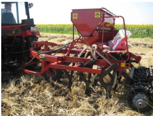
Fig. 3 Seed drill cultivator SCS-2 “Belarus 952”
