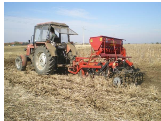
Fig. 4 General view of sowing aggregate and a seed drill cultivator SCS-2
