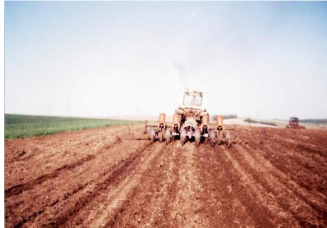
Fig. 4 Sowing maize with simultaneously forming slits with ducts in soil
