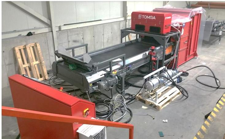
**Fig. 3** Automatic sorting system Finder 1200 chosen for testing
