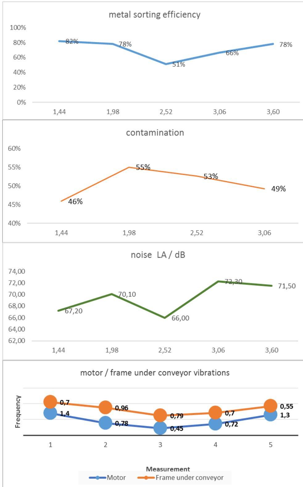
Fig. 5 Graphical illustration of the measured parameters against belt speed
