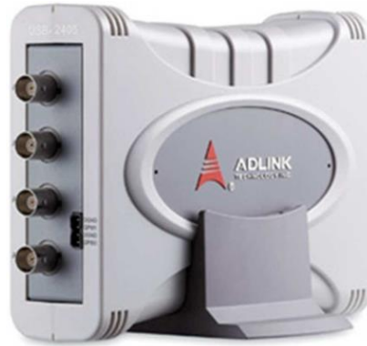
Fig. 2 Adlink USB 2405 signal acquisition module (Adlink 2020)
