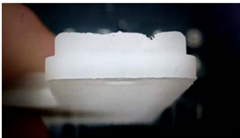
Fig. 3 Imperfectly injected edge of the electronics cover
