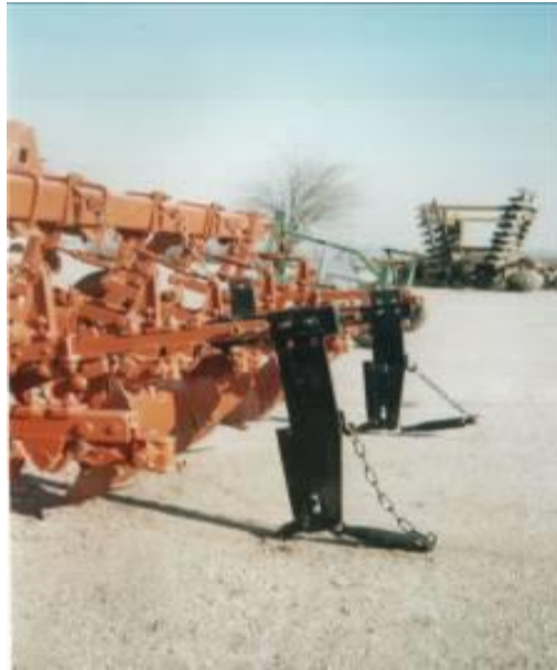
Fig. 7 General view of cultivator KPH-4,2 with a device for soil-breaking with dead-furrowing
