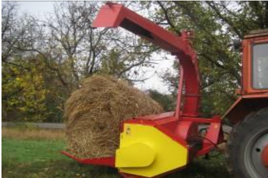
Fig. 9 Universal composting and mulching machine with hydraulic platform
