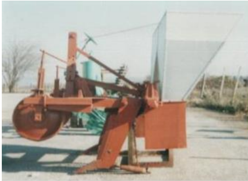
Fig. 1 General view of a modified breaker - dead furrower SHTN-2- 140 with a mulch bunker
