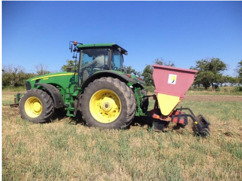
Fig. 4 Device for applying organic matter or mulch to the soil
