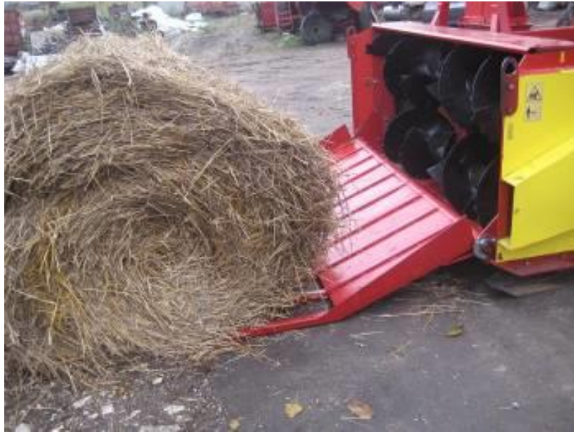
Fig. 11 Hydraulic platform for breaking and shredding round and parallelepiped bales
