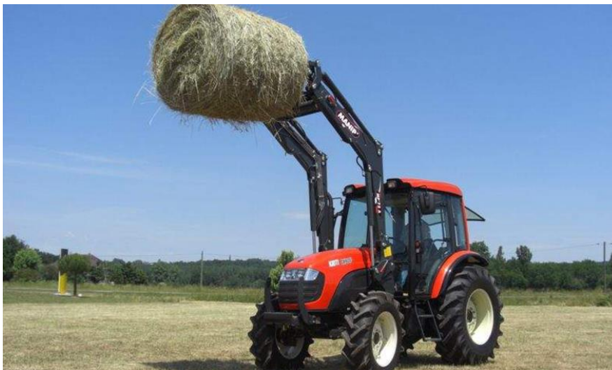
Fig. 12 Front loader with device for round bales and parallelepiped bales
